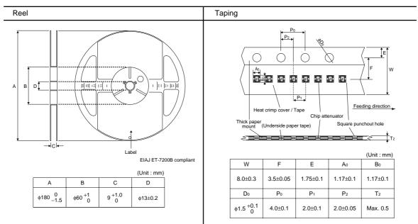
Caution: Insertion direction of device to carrier tape. Marking is on the left bottom side of the cavity to the feeding direction.
